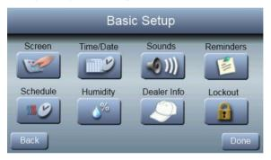
Press **SETUP**; then press **LOCKOUT**. To enable the lockout feature, press the **ON** button. After you have enabled the lockout feature, please select a 4-digit code to be used to unlock the Observer Control. Press **DONE** to return to normal operation.
