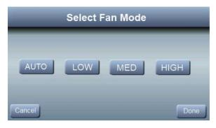
Press **FAN**, then select the desired fan speed; then press **DONE**
