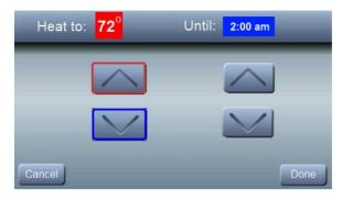
An override time will be displayed on the right side of the screen. You can change the override time in 15-minute increments by pressing the arrows below the time. When you have completed your changes, press **DONE**.
